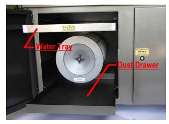
The dust drawer should be cleaned regularly, as needed.
